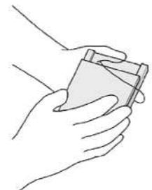
⑤ Keep the short glass plate facing front and slide both plates into the casting frame.
